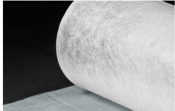
Thin PUR NnF layer on PES support
