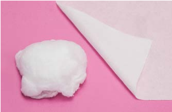
Polycaprolactone nanofibers in 3D cotton-like structure and nanofibrous layer
